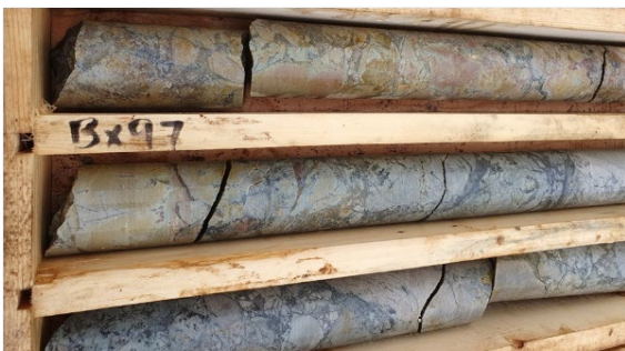
Figure 1: Drill core from ST24-01 from approximately 315.4 – 318m downhole. Dense veins and breccia of visible chalcocite (copper sulfide) can be seen as dark sooty grey, within light grey/tawny dolomite host rocks. This interval also contains blebs of native copper (metallic mineral, top right)
